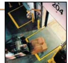
Leveler functions are interlocked with other dock devices to prevent operation until all the safety systems are operational and the dock doors are opened.
